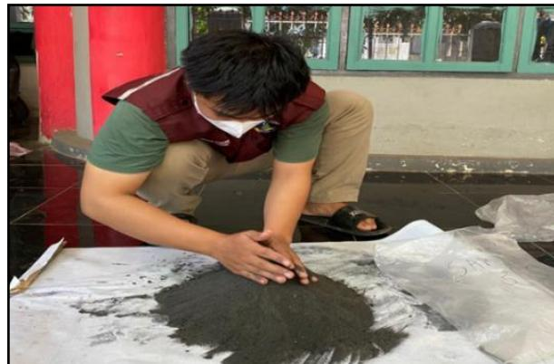
**Gambar 1.** Proses *coning quartering* sampel
